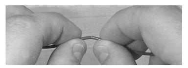
Figure 32 – Separate the buffer tube.
