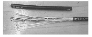
Figure 5 - Remove the 5-inch section to expose the ripcord.
