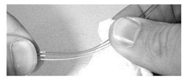
Figure 33 – Clean the optical fibers.
