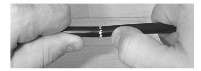
Figure 18 – Flex the cable at the score mark to separate the outer jacket.
