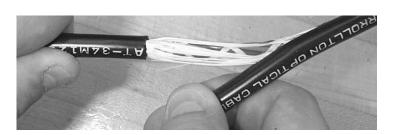
Figure 7 - Remove the outer jacket.
