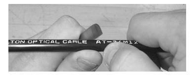
Figure 2 – Ring cut the cable jacket.
