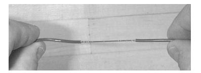
Figure 14 – Remove the buffer tube from the fibers.
