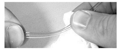
Figure 15 – Carefully clean the fibers.
